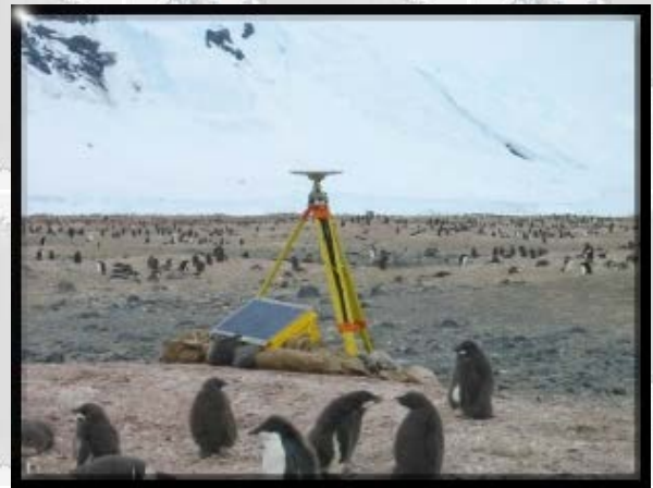
GPS survey of a geodetic control point at Cape Hallett. Photo by Chuck Kurnik.
