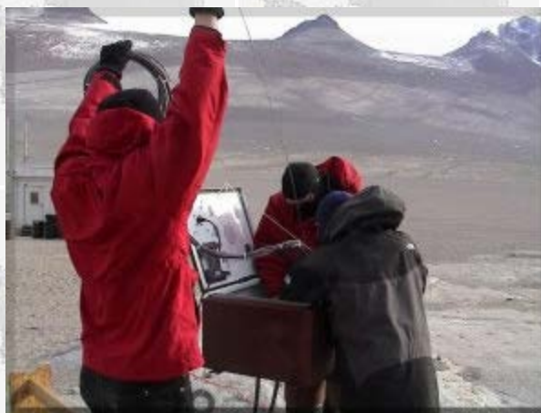
Clay Himmelsbach, Kevin Filiatrault and Will Burk installing a new seismic data digitizing system in a borehole close to Bull Pass in the Wright Valley. Photo by Jimmy Jackson.
