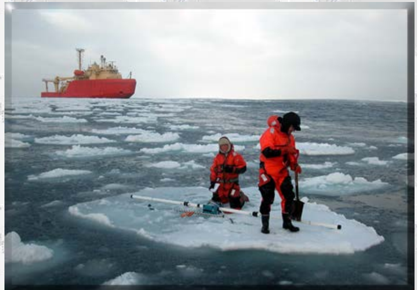
Ice thickness experiment using the EM31 electromagnetic probe on floating first year ice in the Bellinghausen Sea with the R/V Laurence M. Gould in background. Graduate students Nicolas Cullen and Russell Huff wear special waterproof clothing and a Zodiac boat (not seen) is nearby. Photo by Konrad Steffen.
