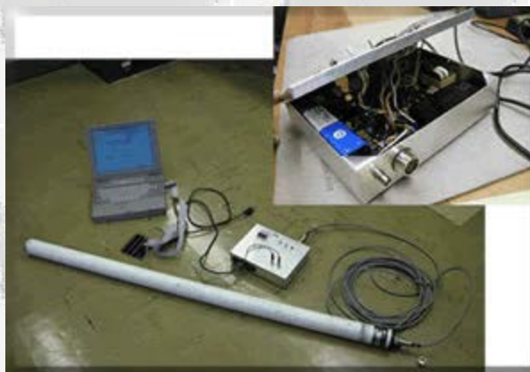
ELF magnetic sensor coil, receiver, and the data acquisition system. Inside the receiver (inset). Photo by Hyomin Kim.
